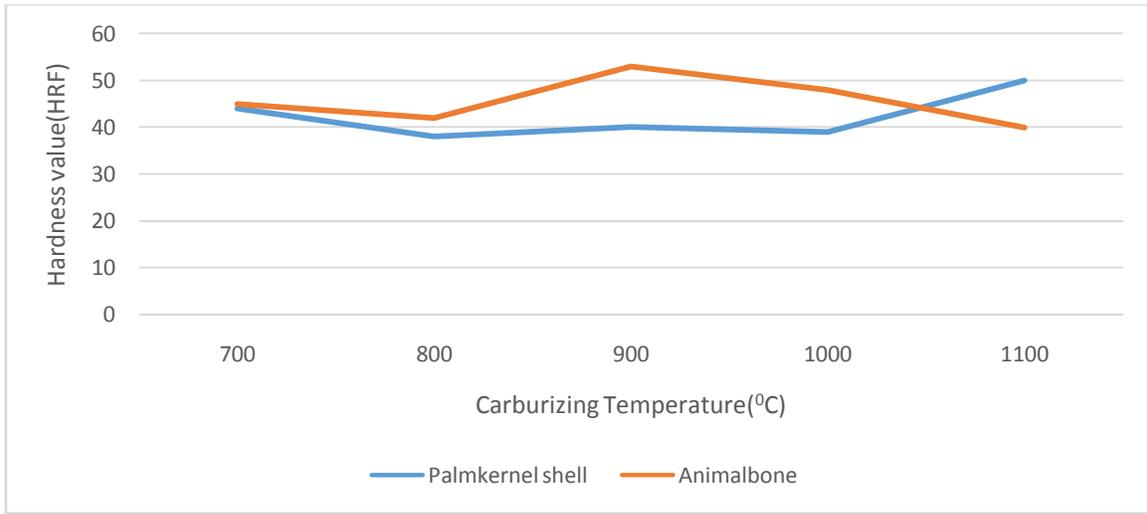
Figure 1: Hardness responses of quenched and tempered samples with carburizing temperature.
