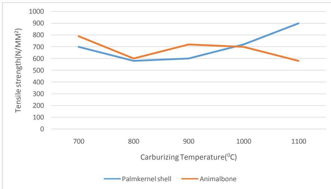
Figure 3: Tensile strengths of carburized, quenched and tempered steel samples with carburized temperature.
