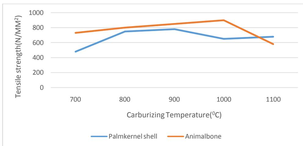
Figure 4: Tensile strengths of carburized, quenched and untempered steel samples with carburizing temperature.
