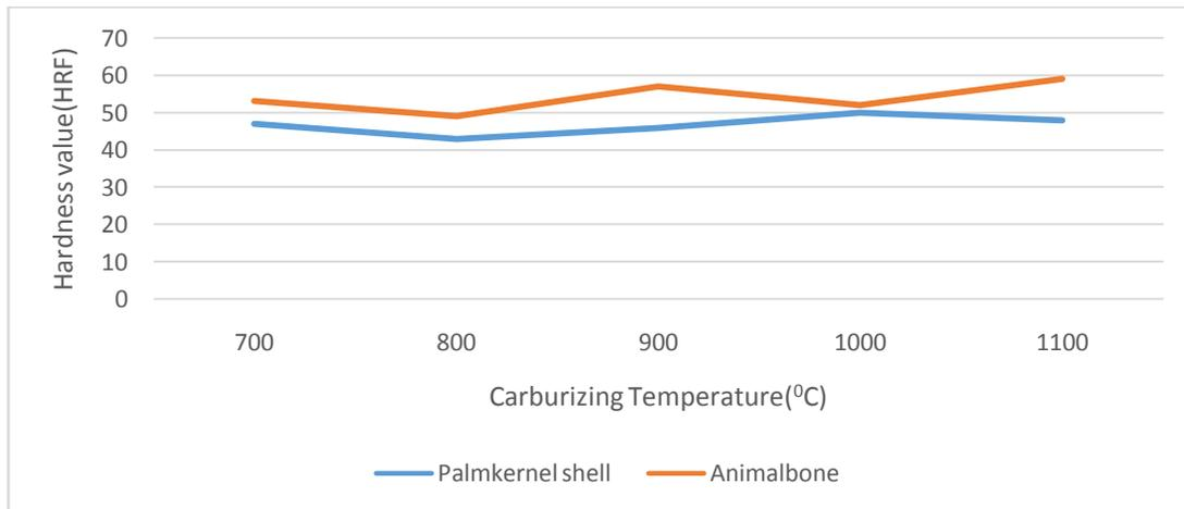
Figure 2: Hardness responses of quenched and untempered samples with carburizing temperature.
