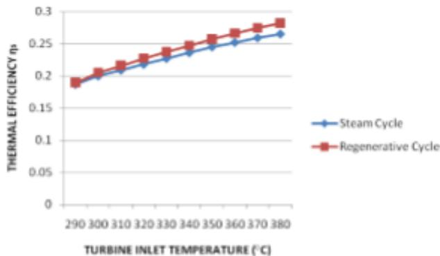
Figure 6: Thermal efficiency vs TIT
