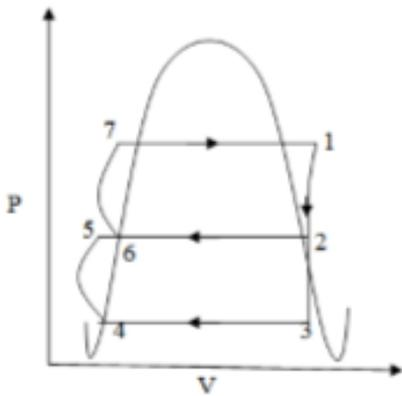
Figure 2: P-V diagram of regenerative cycle
