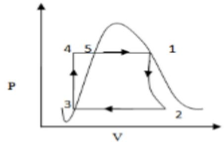
Figure 1: P-V diagram of rankine cycle
