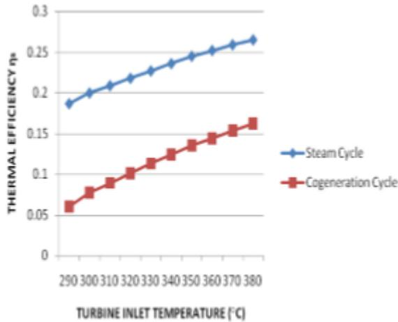
Figure 12: Thermal efficiency vs TIT
