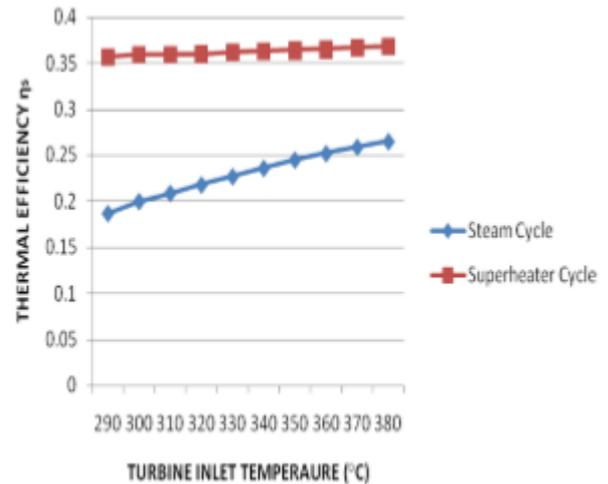
Figure 9: Thermal efficiency vs TIT
