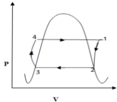
Figure 3: P-V diagram of super-heater cycle
