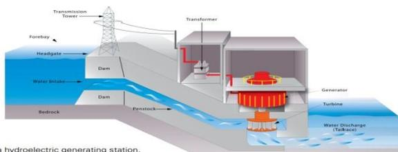
Diagram of a hydroelectric generating station.
