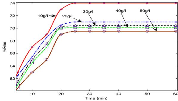
Figure 5: Influence of contact time and varying ADSA dose on the % removal of SDP from BRE (BRE volume =20 ml,  $C_0 = 161.92$  mg/l, initial BRE pH, original temperature =  $25^\circ\text{C}$ ).
