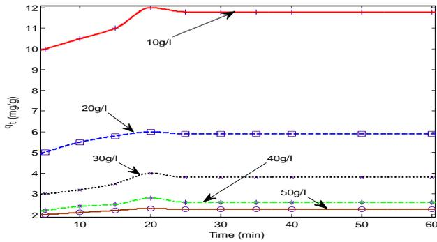
Figure 7: Influence of contact time and varying ADSA dose on the adsorptive capacity (BRE volume =20 ml, C<sub>0</sub> = 161.92 mg/l, initial BRE pH, original temperature = 25°C).
