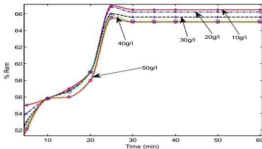
Figure 6: Influence of contact time and varying ADSS dose on the % removal of SDP from BRE (BRE volume =20 ml,  $C_0 = 161.92$  mg/l, initial BRE pH, original temperature =  $25^\circ\text{C}$ ).
