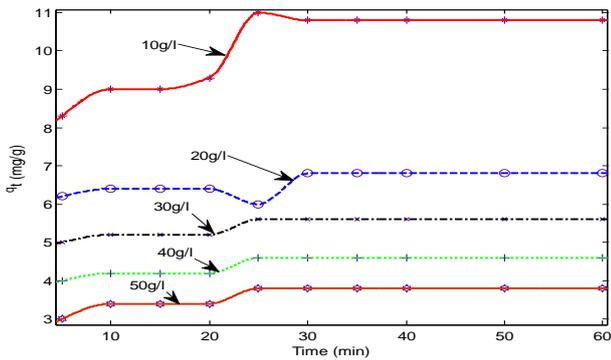
Figure 8: Influence of contact time and varying ADSS dose on the adsorptive capacity (BRE volume =20 ml, C<sub>0</sub> = 161.92 mg/l, initial BRE pH, original temperature = 25°C).
