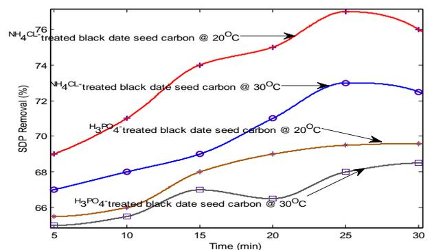
Figure 9: Influence of temperature on the % removal of SDP from BRE onto ADSS and ADSA (adsorbent dose = 50 g/l, BRE volume = 20 ml, C<sub>0</sub> = 161.92 mg/l, initial BRE pH, contact time = 30 min).
