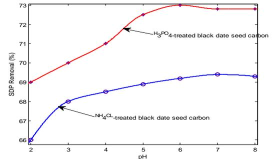
Figure 11: Influence of pH on the adsorption of SDP from BRE on to ASAS and ADSA (adsorbent dose = 50 g/l, BRE volume = 20 ml, C<sub>0</sub> = 161.92 mg/l, Temperature 30°C, contact time = 30 min).
