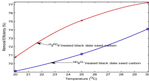
Figure 10: Influence of temperature on removal efficiency of SDP on to ADSS and ADSA at contact time of 30 min (adsorbent dose = 50 g/l, BRE volume = 20 ml, C<sub>0</sub> = 161.92 mg/l, initial BRE pH).
