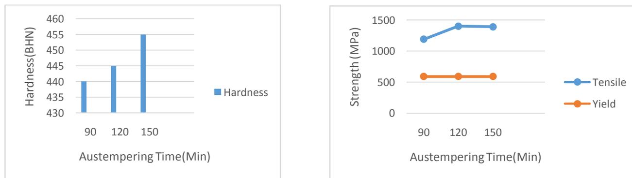
**Figure 4 (a)** Mechanical Properties of produced ADI at 300°C at different Austempering Time
