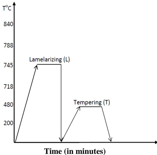
Figure 3: Temperature – Time graph involving Lamellarizing and Tempering (L+T)
