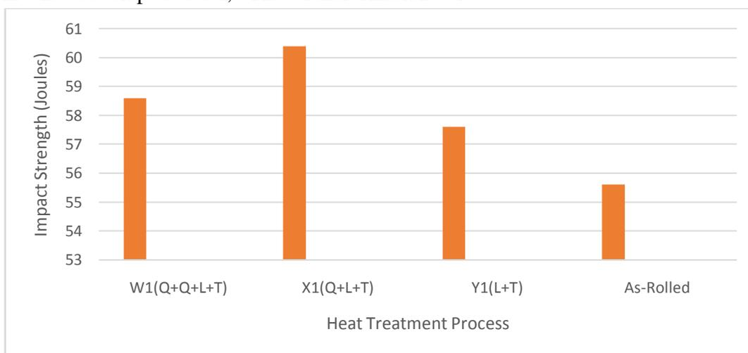
**Figure 8: Impact Strength of Heat Treated Specimens and As-Rolled Medium Carbon Steel.**
