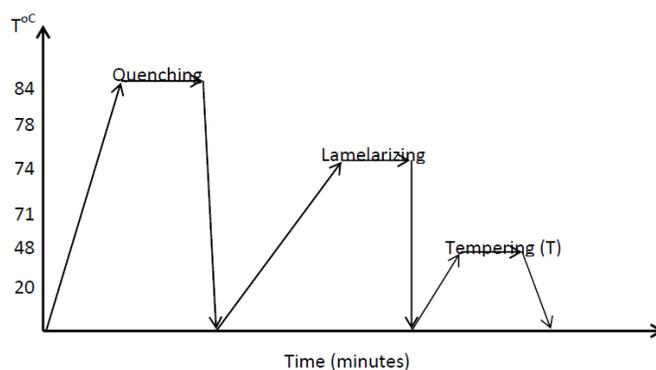
Figure 2: Temperature – Time Graph involving Quenching Lamellarizing and Tempering (Q+L+T).
