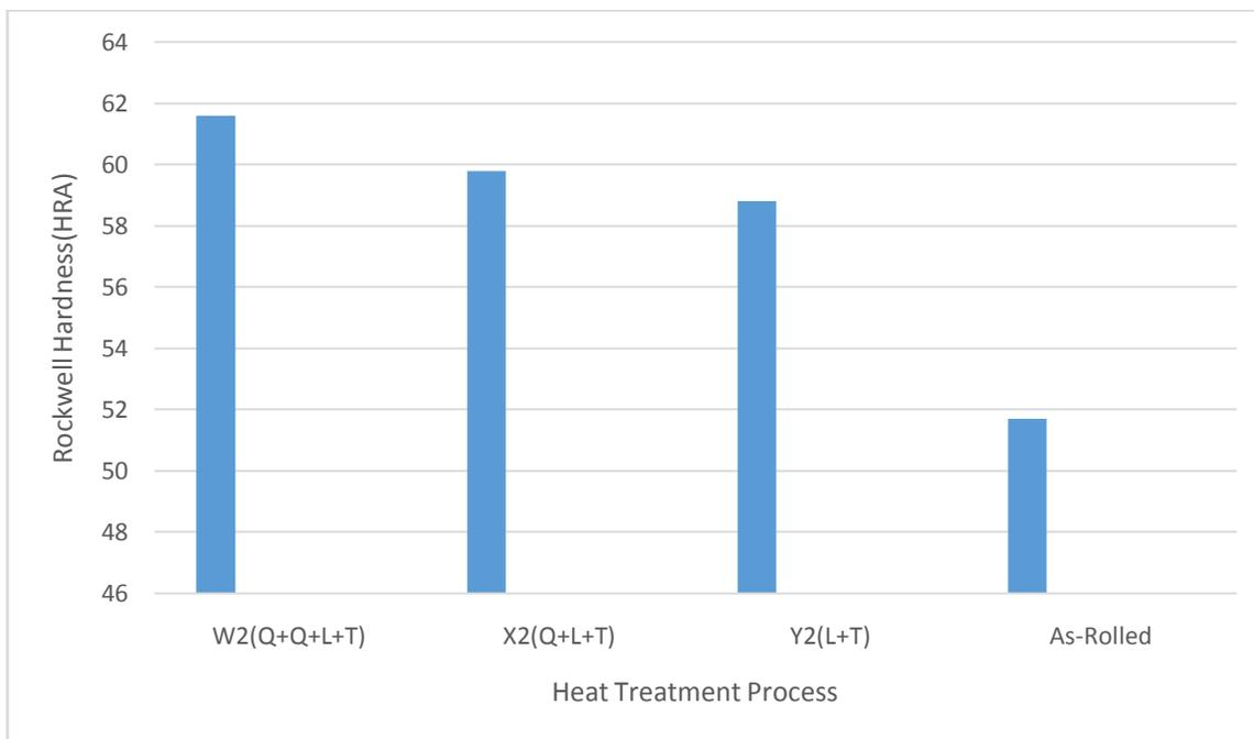
**Figure 7: Rockwell Hardness number after various Heat Treatment Processes**
