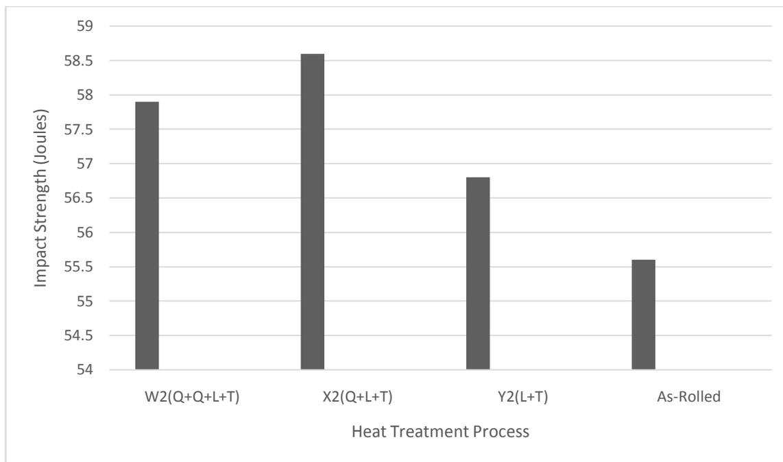
**Figure 9: Impact Strength of Heat Treated Specimens and As–Rolled Medium Carbon Steel**
