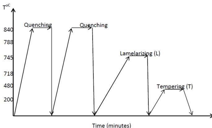
Figure 1: Temperature – Time Graph involving Quenching, Quenching Lamellarizing and Tempering (Q+Q+L+T).
