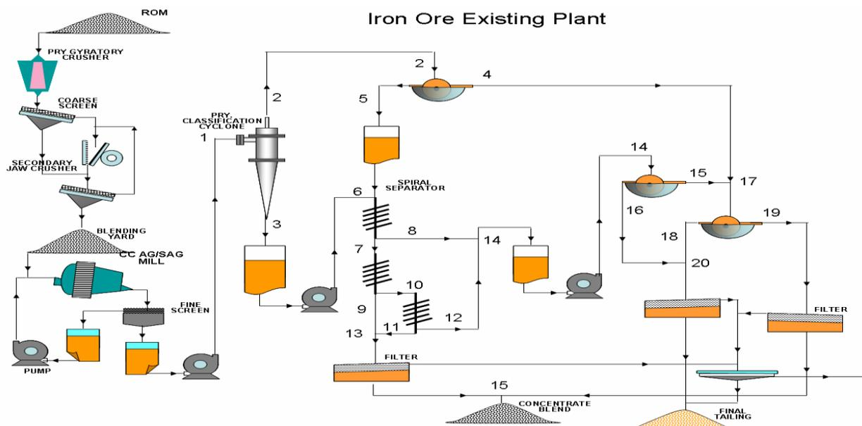
Figure 1: Simplified process flowsheet of Itakpe iron ore processing plant
