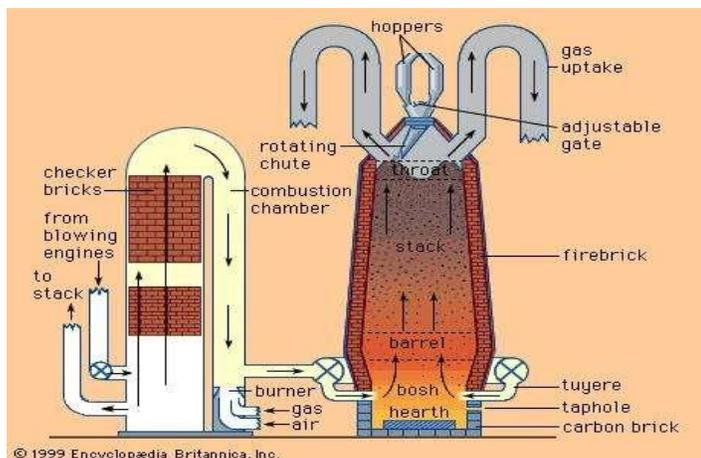
Figure 3: Schematic diagram of modern blast furnace (right) and hot-blast stove.
