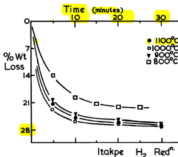
Figure 2: Isothermal mass change data for  $H_2$  reduction of Itakpe Ore
